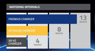
Conditions: The topping up intervals are based on 80%DoD - 5 cycles per week The following charging factors are considered:
