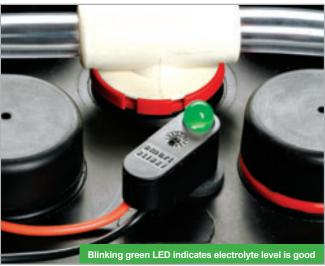
Philadelphia Scientific's battery watering monitors' compact size allows fit onto crowded battery tops and their very bright LED allows for maximum visibility.
