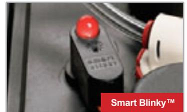
Smart Blinky's are available with standard indication sequence or 5 day delay. The 5 day delay option sensors when the electrolyte has gone below the level of the probe, with the LED only turning red after 5 days. This option enables you to increase further the intervals between watering.
