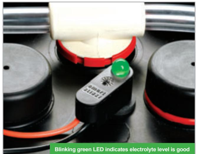
Blinking green LED indicates electrolyte level is good
