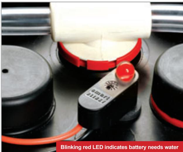
Blinking red LED indicates battery needs water
