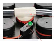
risk of damage caused by battery cables (1.10 in. or 2.79 cm)
